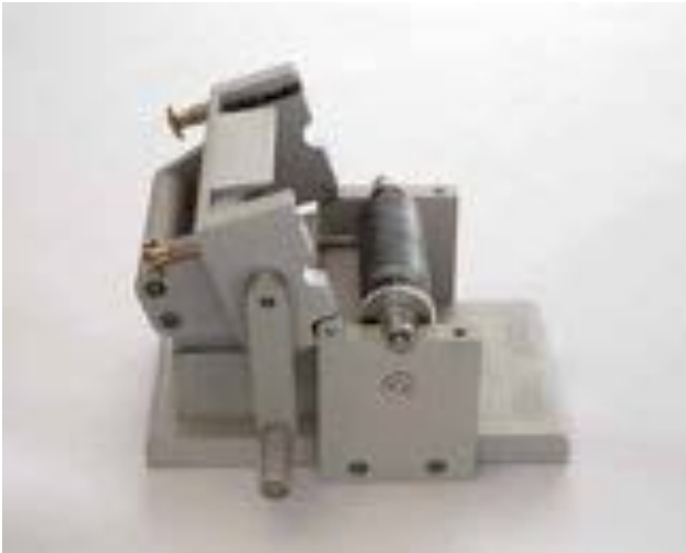
Bridge opened for cleaning and access to the cutting axis
